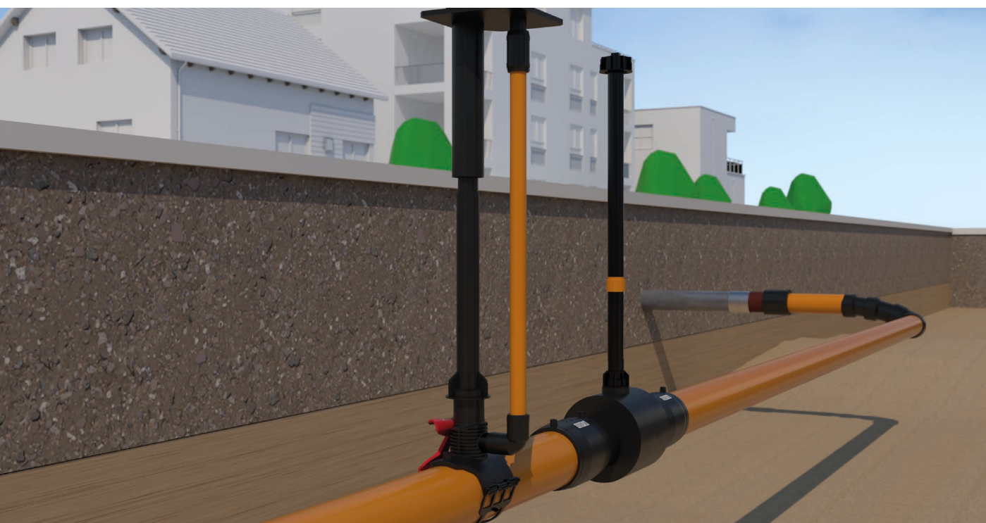
The combination of ball valve and purge stack GAB
